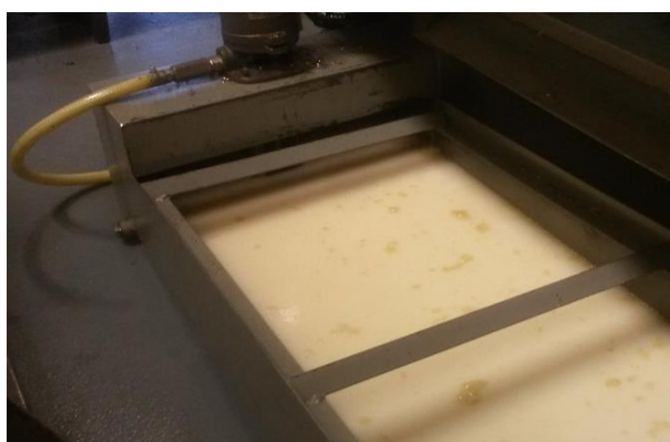
Fig. 1 Cooling system of the turning machine CHEVALIER FC-2140
